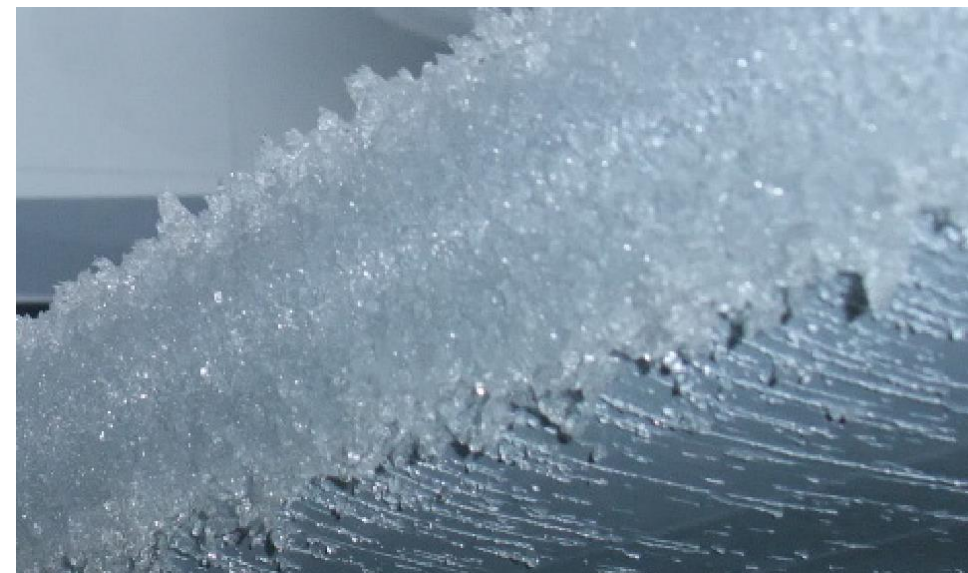
Ice accretion on wing leading edge
