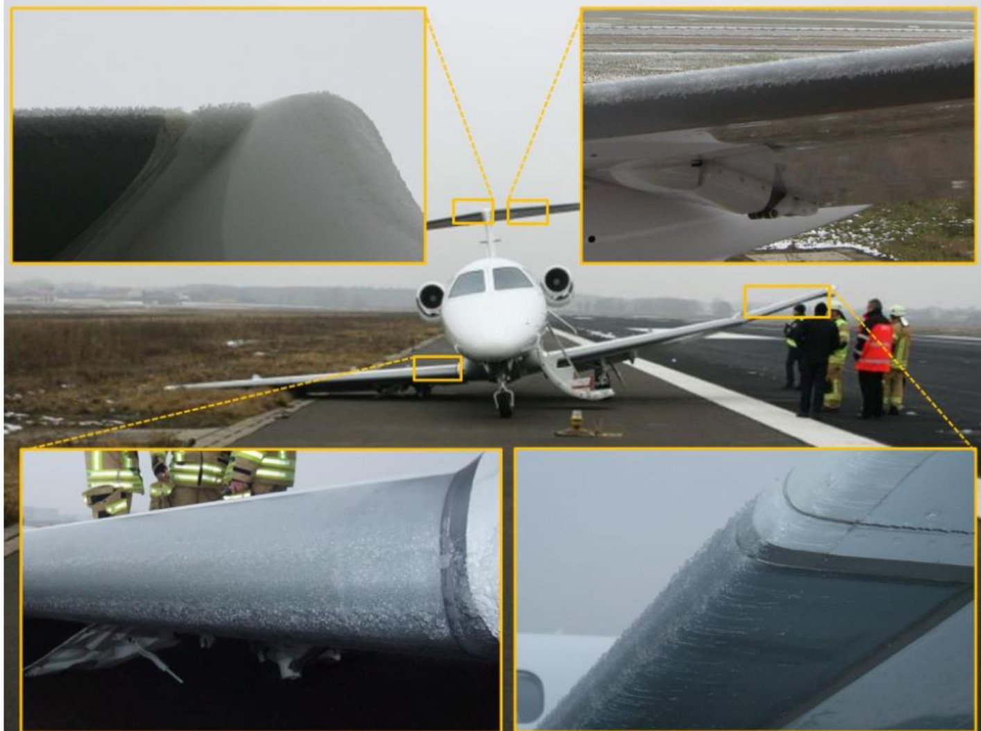
Ice accretion on wing leading edge
