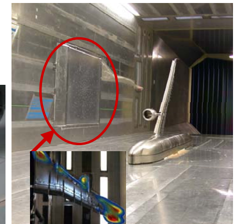
Low Reynolds number testing including acoustic array
