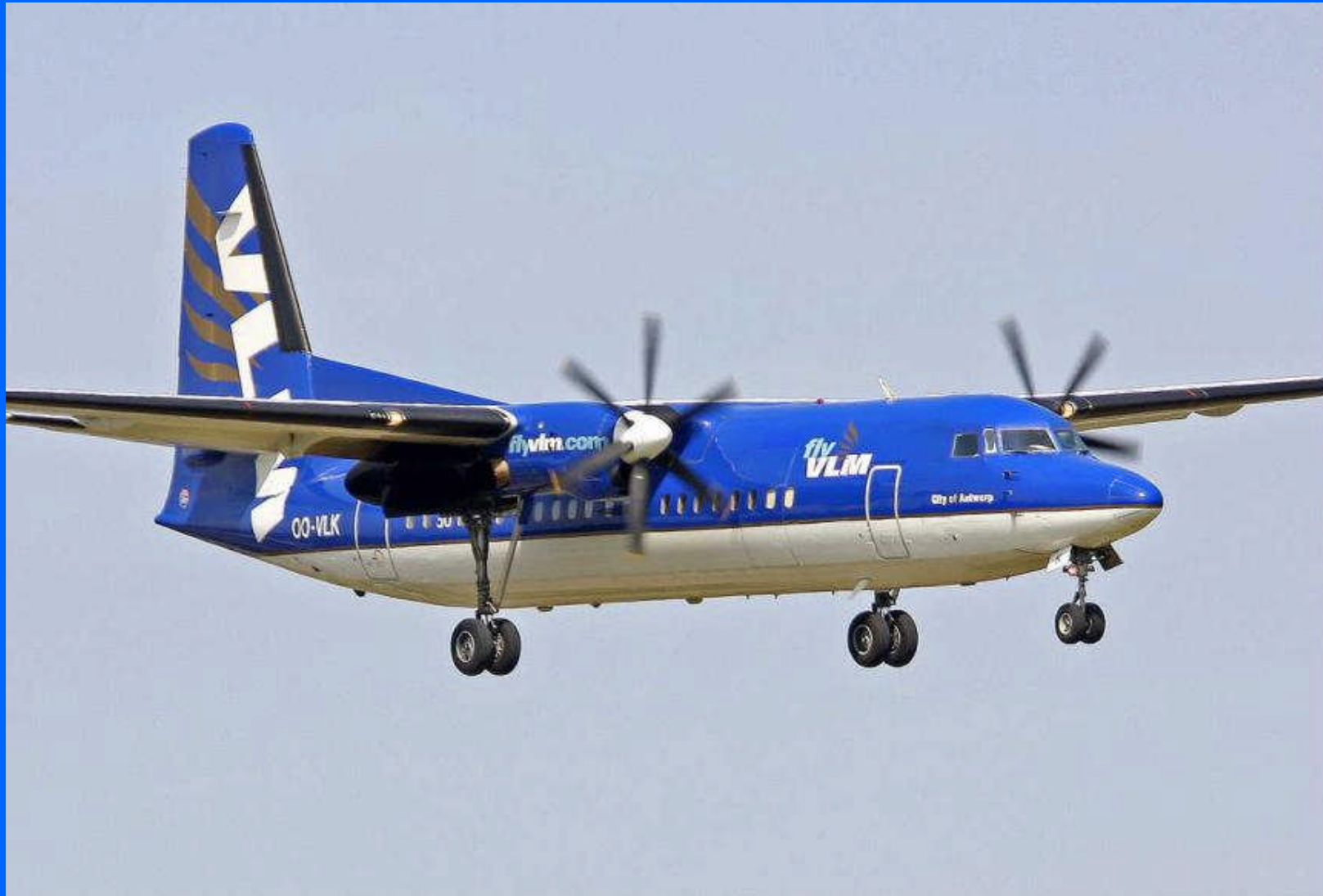
Fokker 50 with Dowty computer-controlled 6-bladers
