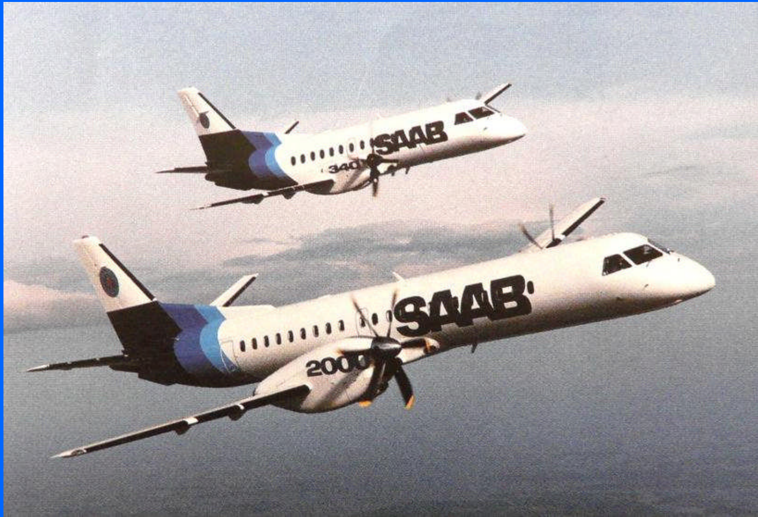
Saab 2000 High-speed Turboprop - 1992 Dowty 6-blade swept propellers with integrated electronic control
